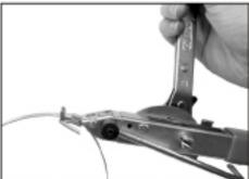
Form a clamp by threading the band through buckle and make a fold under the buckle. Insert tail of clamp into head of tool and slide into slot of winding mandrel. Depress locking pawl and tension clamp with forward strokes of the ratchet wrench.
