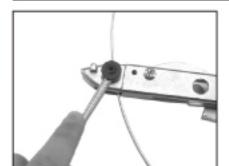
Cut off adequate band from roll of 1/4" or 3/8" BAND-IT band by opening the slot in the head of the tool with the cut off lever at right angles to the tool. Thread the band through the slot and
