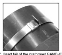
7. Insert tail of the preformed BAND-IT Jr. clamp into the tool. Tension as shown in steps 2 & 3. When tensioned sufficiently, release locking pawl and rotate over object being clamped. Cut off, leaving stub.
