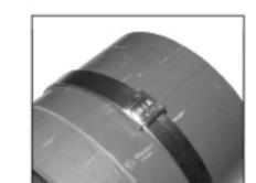
Complete clamp by tapping lip of band over buckle and remove ratchet wrench from tool as shown in step 6.
