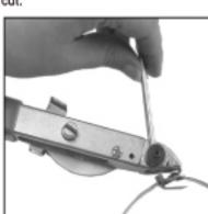
Cut off excess band by lifting cutter
